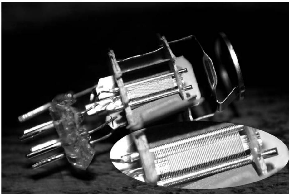
Figure 27 - Internals of 12AX7 valve with anode structure cut away to reveal detail of cathode arrangement and surrounding grid
