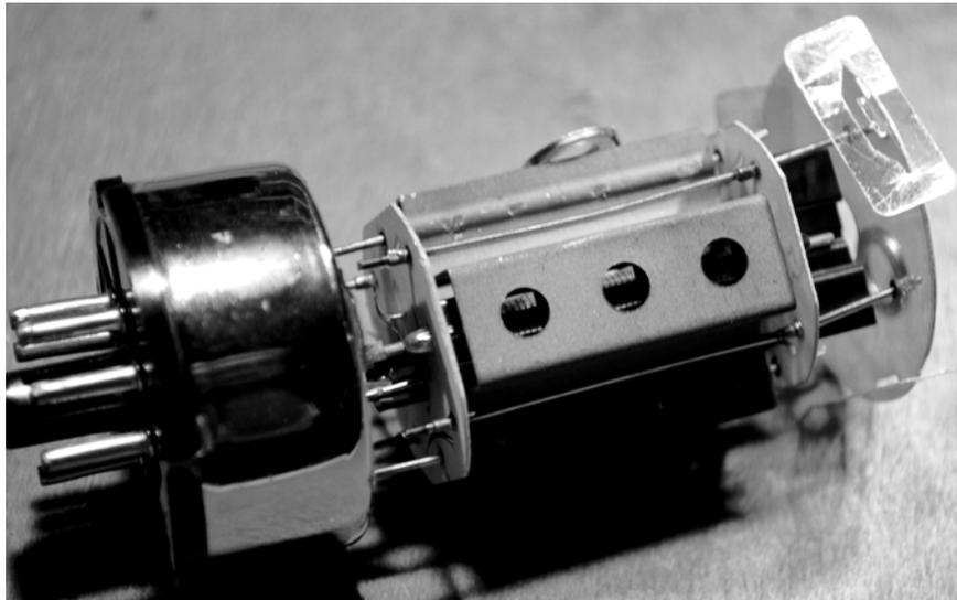
**Figure 28 - KT100 (KT88) valve with glass envelope removed**
