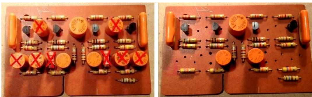
**Figure 1 - Modifications to the disc preamplifier board (M12019)**
