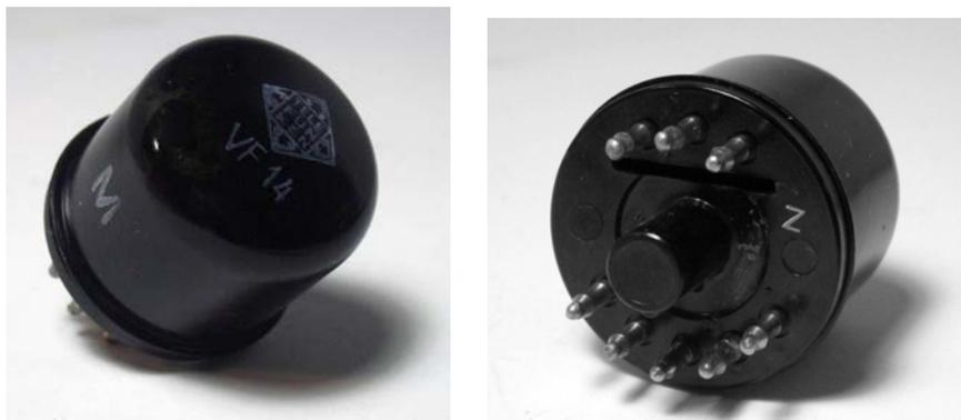
Figure 36 - The VF14 valve used in the impedance converter of the U47
