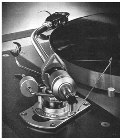
Figure 7 - By cranking the pickup head in relation to the axis of the tone-arm and in arranging the stylus point to pass in front of the turntable centre the pickup stylus and the groove tangent is reduced to plus/minus a few degrees across the recorded groove.
