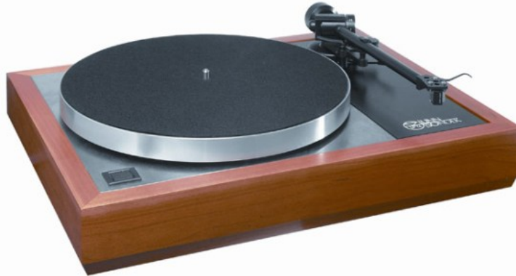
Figure 5 - The Linn Sondek, a famous high-end record-player incorporating a suspended, mechanically and acoustically isolated sub-chassis for the tone-arm and turntable and belt drive from an (optionally) crystal-controlled high-quality motor. The turntable is supported on a single-point bearing for minimum rumble .
